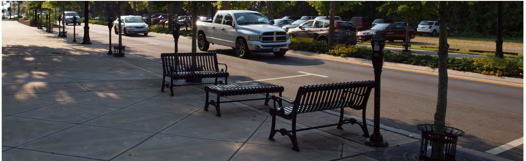
Example of streetscape using benches and trees to buffer pedestrian space from vehicular roadway.
