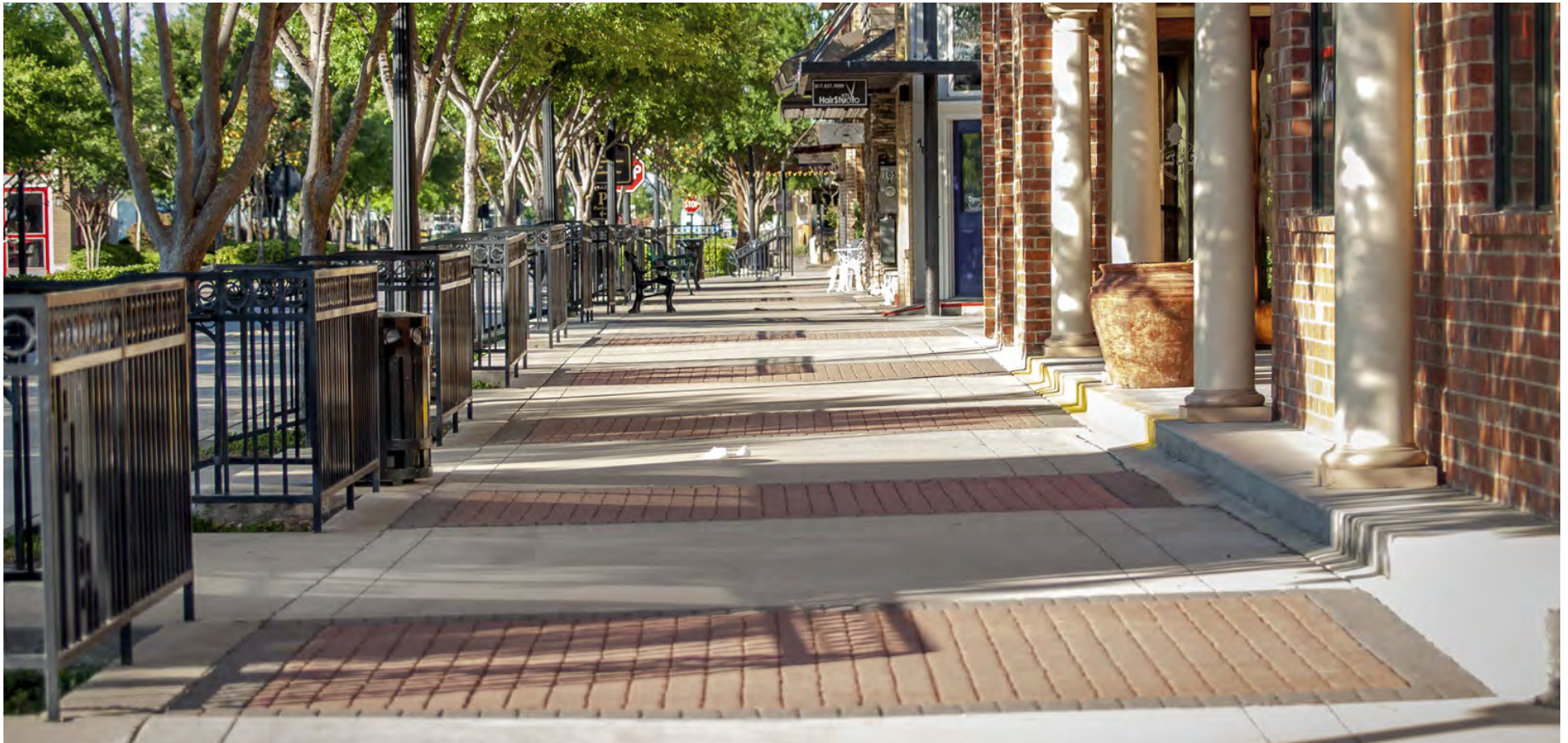
Pavement can be used to define spaces through use of color, texture, pattern and material.
