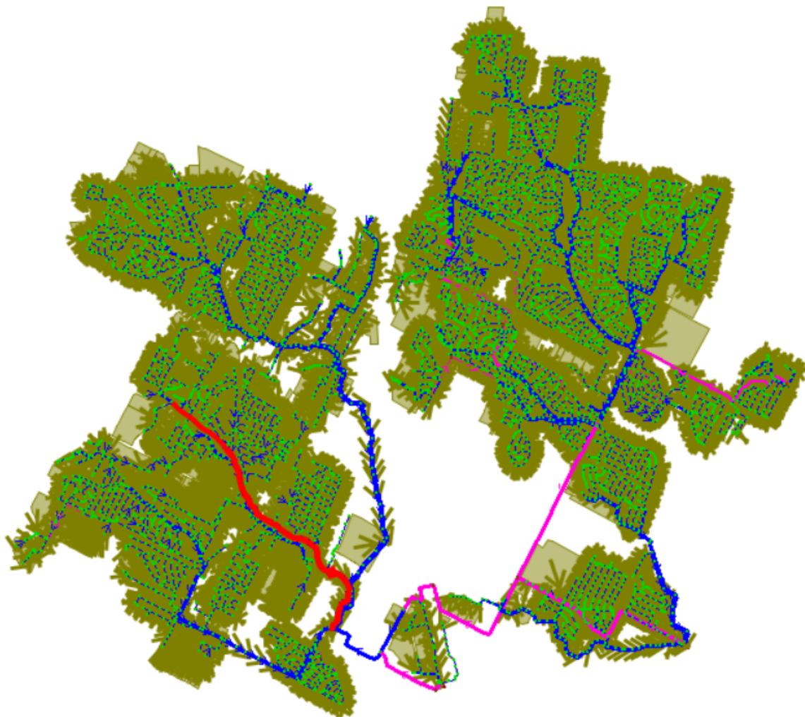
Figure 5-3. InfoWorks ICM Downstream Network Trace
