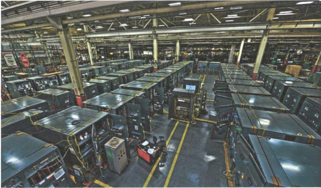
Above: 99 sections of Cummins MV Paralleling Switchgear factory tested as a complete system
