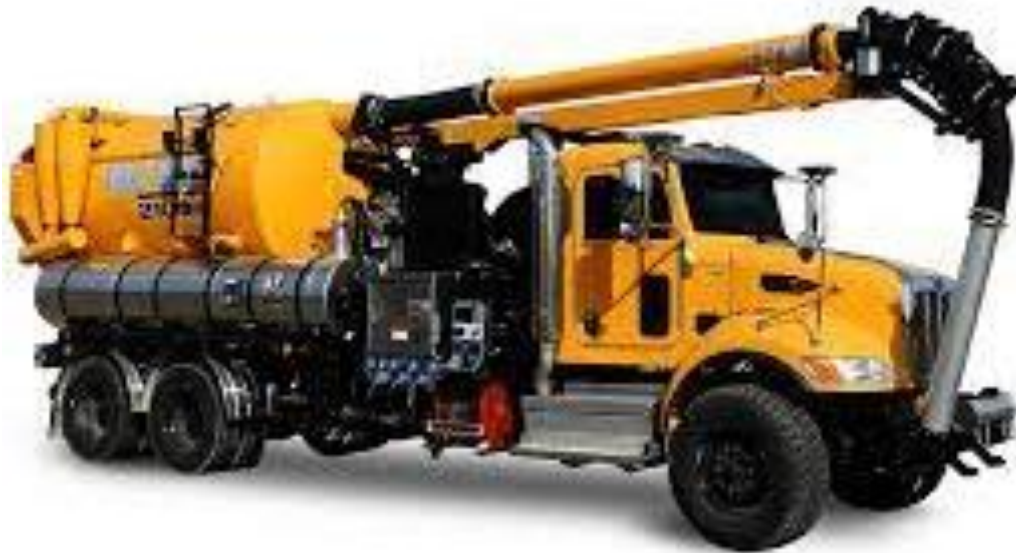
2100i Catch Basin Cleaner/Hydro Excavator
