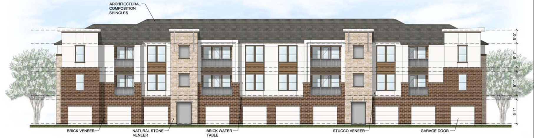
TYPICAL BUILDING ELEVATION - INTERIOR DRIVE
