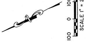
ALL BEARINGS ARE BASED ON GRID BEARINGS. DISTANCES ARE SURFACE DISTANCES. COORDINATES ARE SURFACE VALUES BASED ON THE TEXAS STATE PLANE COORDINATE SYSTEM, NAD 83, CENTRAL TEXAS ZONE USING A COMBINED SURFACE ADJUSTMENT FACTOR OF 0.999990000.
