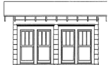
This grouping is commonly found in dormers. As size accentuates, the window width also becomes one-third of a dormer.
