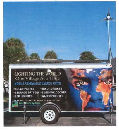
MoRE<sup>TM</sup> provides self contained, easily transported light, power and solar cooking on wheels.
