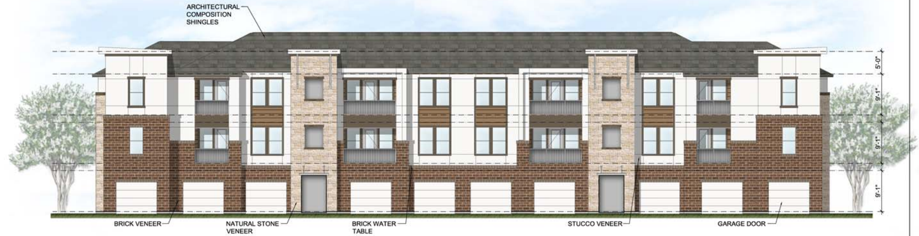
TYPICAL BUILDING ELEVATION - INTERIOR DRIVE
