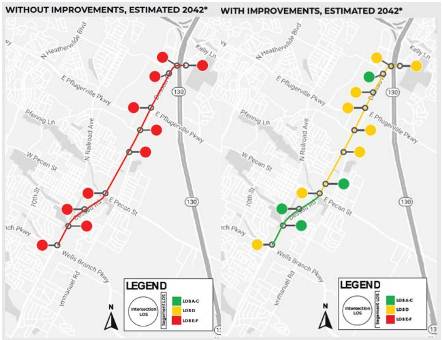
Figure 6-15: LOS in 20 Years With and Without Improvements
