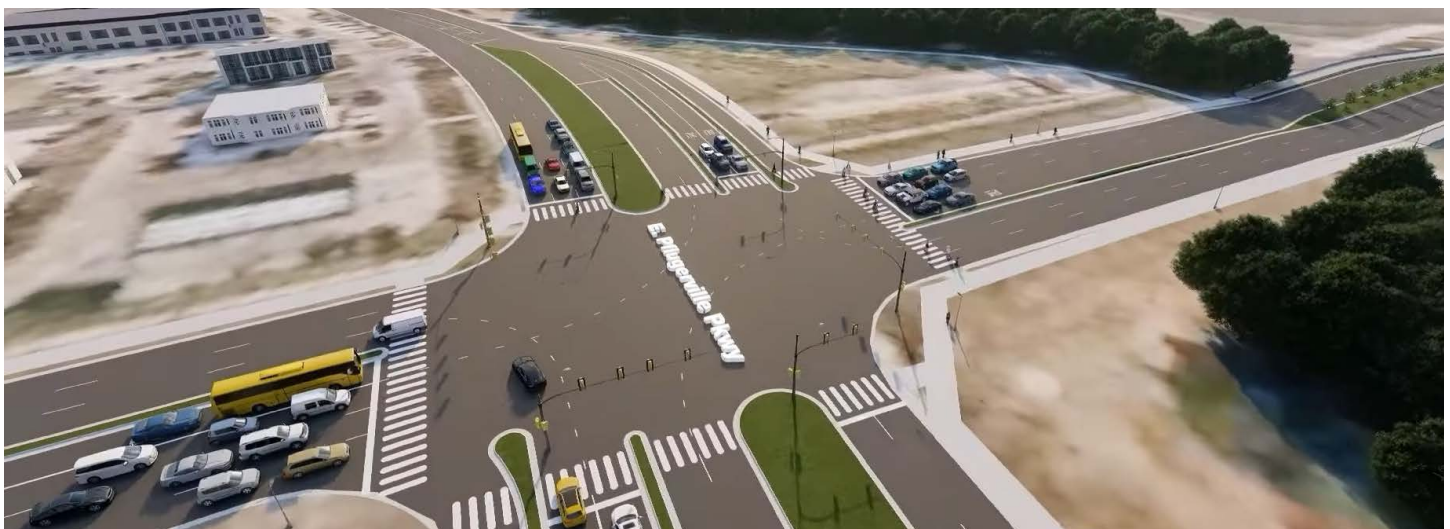
Figure 6-2: 3D Rendering of E. Pflugerville Pkwy Continuous Flow Intersection
