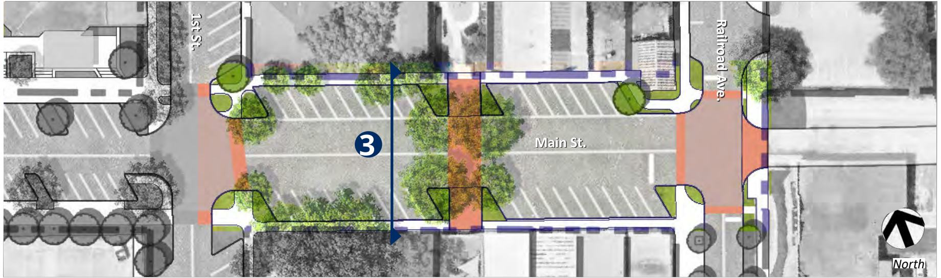
Plan view of proposed Main St. improvements between 1st St. and Railroad Ave.
