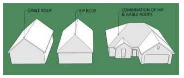
3. Pitched Roof Type and Material Standards. Tile, metal or asphalt shingles (laminated 320-pound, 30-year architectural grade asphalt shingles or better) shall be the dominant roof material. Any other roofing material not stated shall not be permitted unless approved by the Planning Director.
