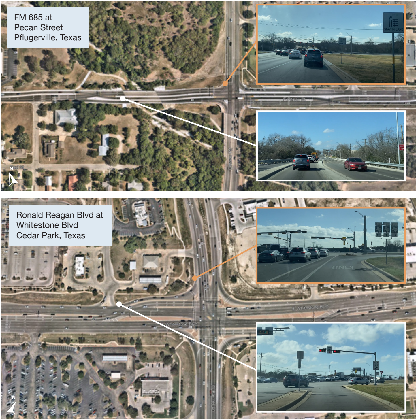
Figure 6-11: Continuous Flow Intersection Comparison
