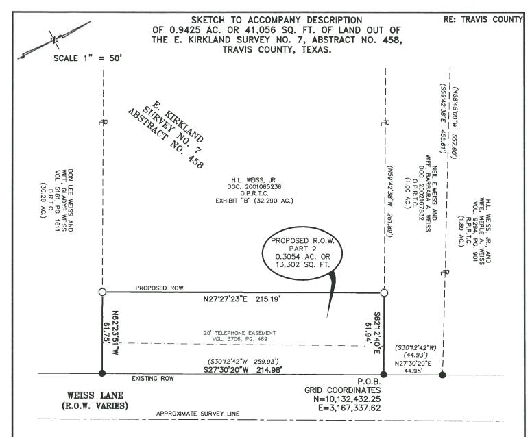
1. THE COORDINATE SHOWN HEREON IS BASED ON THE TEXAS STATE PLANE COORDINATE SYSTEM, CENTRAL ZONE, NAD83 (CORS96) DATUM AND WAS ESTABLISHED BY GPS OBSERVATION. THE BEARINGS SHOWN ARE GRID BEARINGS. THE COMBINED GRID TO SURFACE SCALE FACTOR IS 1.00010. ALL DISTANCES SHOWN ARE SURFACE DISTANCES.
