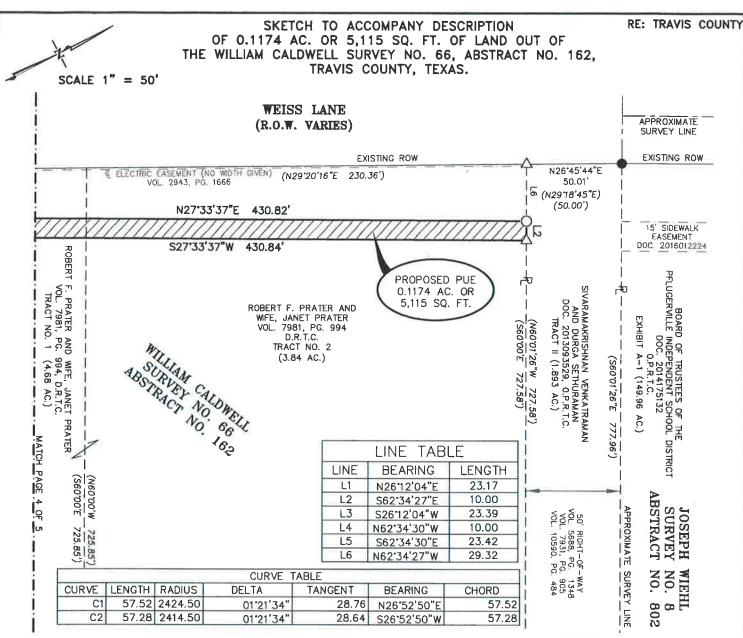
1. THE COORDINATE SHOWN HEREON IS BASED ON THE TEXAS STATE PLANE COORDINATE SYSTEM, CENTRAL ZONE, NADB3 (CORS96) DATUM AND WAS ESTABLISHED BY GPS OBSERVATION. THE BEARINGS SHOWN ARE GRID BEARINGS. THE COMBINED GRID TO SURFACE SCALE FACTOR IS 1.00010. ALL DISTANCES SHOWN ARE SURFACE DISTANCES.
