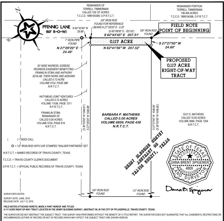
THE BEARINGS SHOWN HEREON ARE BASED UPON THE TEXAS STATE PLANE COORDINATE SYSTEM, NAD 83, TEXAS CENTRAL ZONE ACQUIRED FROM GLOBAL POSITIONING SYSTEM OBSERVATIONS.
