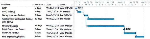
Based on the schedule, HVJ has tentatively scheduled the FWD testing the Friday following the NTP. The ability to perform the FWD field work within 2 days of the NTP will require City approval of field testing plan including traffic control. There is some cushion for weather, but no major weather delays.
