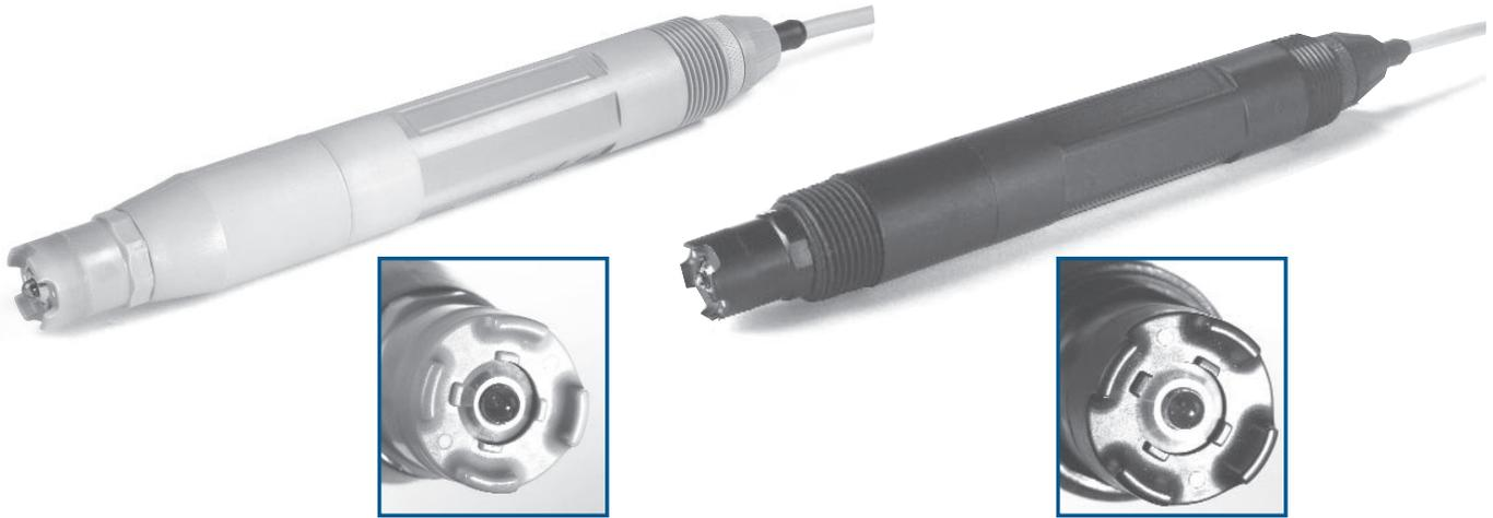
Hach Digital pH/ORP sensors are available in convertible (PEEK® or Rytion®), insertion, and sanitary body styles. Three electrodes are used in these sensors to increase measurement accuracy and eliminate sensor ground loops.
