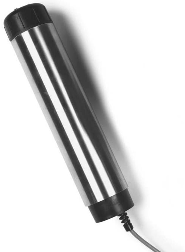
*Break-through luminescent technology for dissolved oxygen. The HACH LDO<sup>®</sup> Dissolved Oxygen Probe continuously monitors DO with this revolutionary method of detection. It's virtually maintenance-free with no membranes to replace, no electrolyte solution to replenish, and no anode or cathode to clean or replace.*
