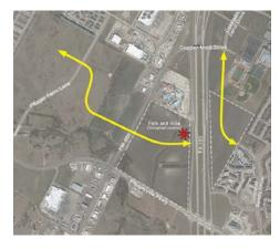
through the proposed West Tract to provide a connection from FM 685 to the SH 130 Frontage Road. The PUD includes a cross section for the segment of Geraldine Drive which includes two travel lanes with a turn lane, designated on-street parallel parking lanes, and wide sidewalks.
