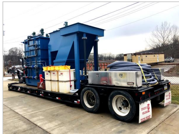
Figure 3 Front view of the plate settler pilot
