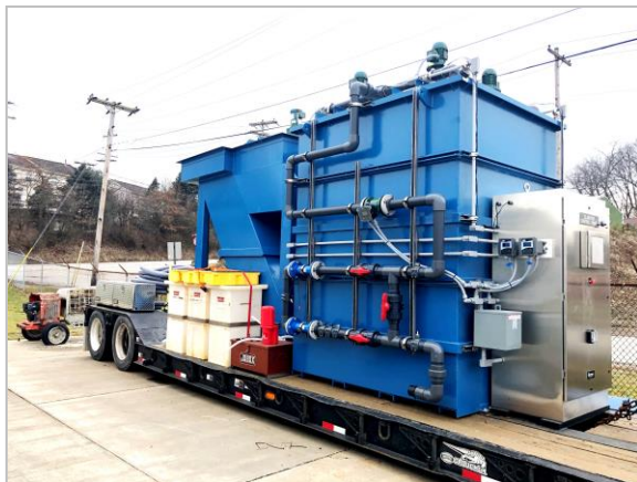
Figure 3 Front view of the plate settler pilot
